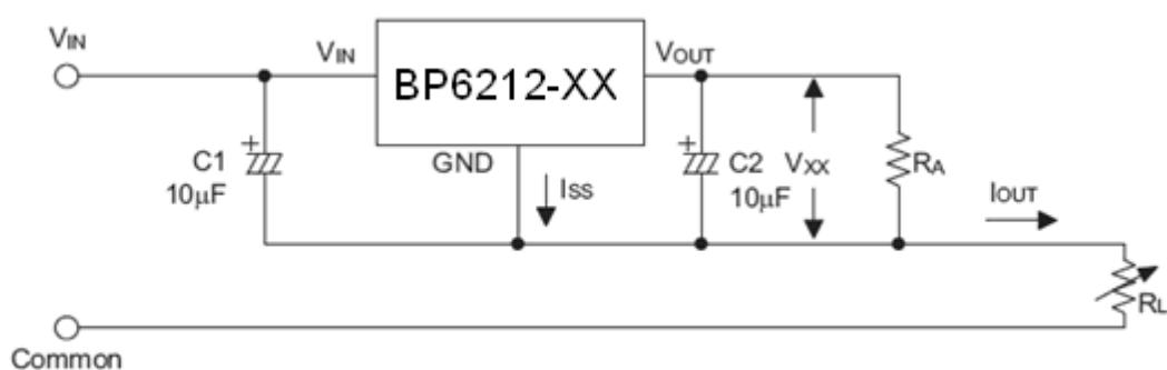
$$I_{OUT} = \frac{V_{xx}}{R_A} + I_{ss}$$
